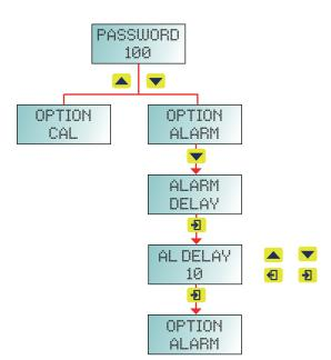
The X5 allows you to set an alarm delay of up to 99 seconds. The default value is 10 seconds.
