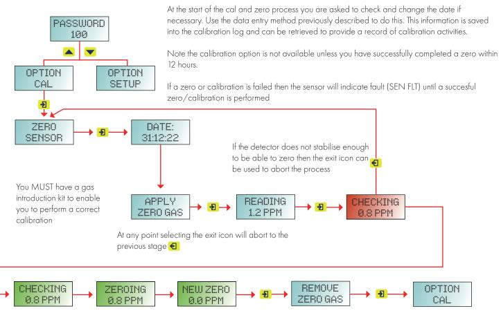
The process allows the engineer to observe the state of the existing zero, perform a zero and then observe the results. Ensure readings are back to normal levels before exiting the menu system. Whilst in the menu system alarms are inhibited. Ensure readings are back to normal levels when observing at the 'NEW ZERO' stage before progressing.
