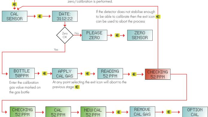
The process allows the engineer to observe the state of the existing calibration, perform a calibration and then observe the results. Ensure readings are back to normal levels before exiting the menu system. Whilst in the menu system alarms are inhibited. Ensure readings are back to normal levels when observing at the 'NEW CAL' stage before progressing.
