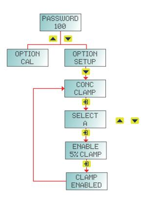
The concentration clamp setting is either on or off for either port A or B.
