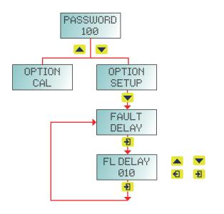
Use this menu item to set the delay period in seconds before the fault relay/indication activates.
