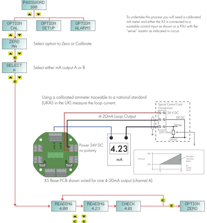
The mA zero or cal option both work in the same manner. Select Option Zero or Option Cal from the menu. For option zero the X5 will generate 4mA based on its last zero. With a mA meter connected as indicated in the enclosed diagram use the icon buttons to enter meter reading as displayed. When entered the screen shows 'check' and displays the newly corrected mA output value. You then have the option to abort and go through the process again or continue and return to the 'option' menu selection.
