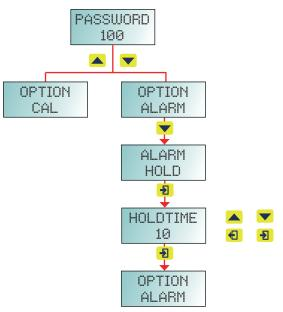
The X5 allows you to set a hold time for alarm relays of up to 255 seconds. In operation when an alarm level resets, either automatically or on user action, the unit then stays in alarm until the hold time period expires.
