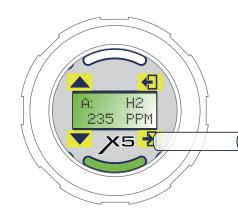
To enter the menu system hold the magnetic wand over the ENTER symbol for at least 5 seconds.
