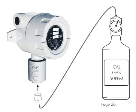
Response time of the detector can be tested using a stopwatch to check the time for the detector to reach 90% of the applied calibration gas value from first application of the calibration gas.
