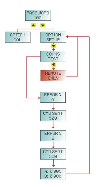
The comm's or communications test is used to test the quality of serial communication when detectors are connected remotely from the X5.
