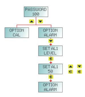
Alarm levels can be adjusted from the default pre-sets. In the option menu select either set AL1 or set AL2 as desired. The existing alarm level is displayed, note that units are not shown. You will not be able to set an alarm level outside of the detector range. Use the data entry method to set the new alarm level and enter. The display returns to the option setup menu.
