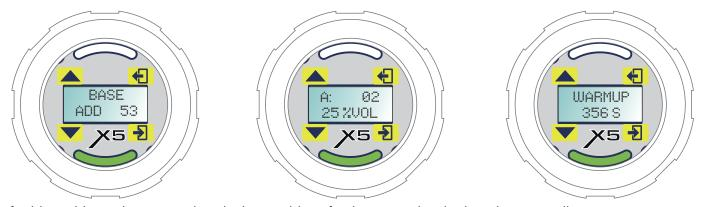
If addressable mode is active then the base address for the unit is also displayed sequentially. The display then indicates the warm up time, this is variable depending on the detector type. After the warm up time the display sequentially shows each detector and its readings.
