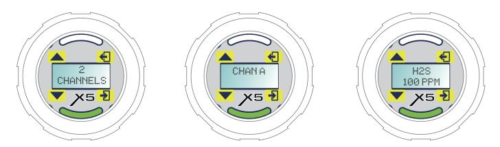
The status indicator stays green if the gas detectors are connected otherwise a channel fault is indicated for the affected channel. The display shows the number of channels and then their type and range.
