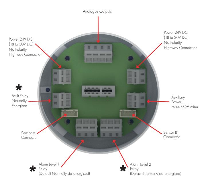
Note relays are rated for 12/24V DC Operation at up to 4A
