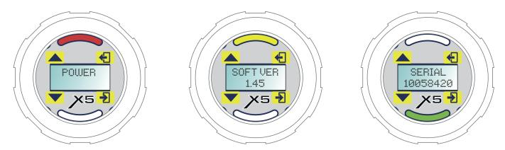
On power up the display back light will show blue with the status indicators cycling red, yellow, green. The display shows the software version and serial number.
