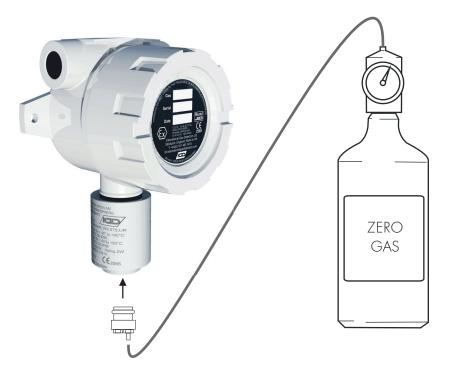
Gas calibration kits are available for purchase. They include fixed gas flow regulators to deliver test gases at the correct flow rate and calibration caps. It is imperative to have the correct flow rate and to use the correct calibration cap.
