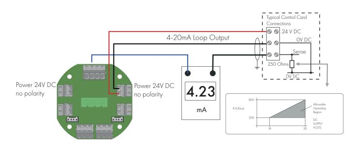
X5 Base PCB shown wired for one 4-20mA output (channel A) Note Power can be applied to either of the two available power connectors.
